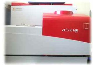
Differential Scanning Calorimeter
